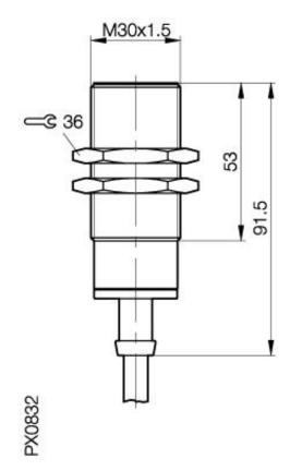
Inductive Sensors BES 516-120-SA2 M30x1.5 x 87 Complementary Sn=10mm shielded temperature rated
